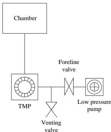
Fig. 1 Schematic diagram of vacuum system.
