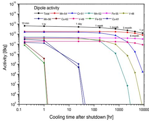
Fig. 4. Activities in the dipoles according to the cooling time after an irradiation of 3000 hours
