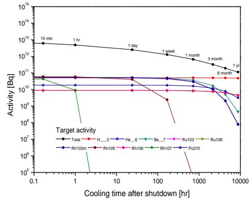
Fig. 7. Total activity of pre-separator according to the cooling time after an irradiation of 3000 hours
