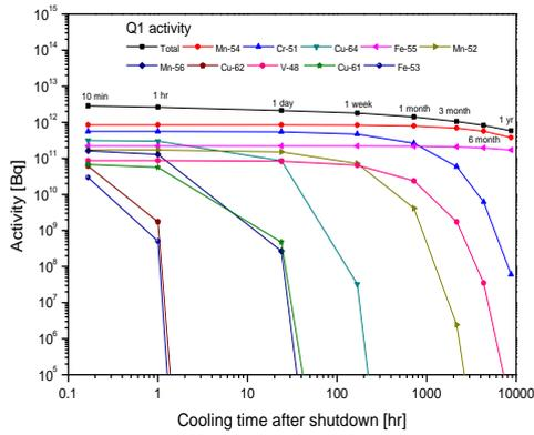
Fig. 5. Activities in the quadrupoles according to the cooling time after an irradiation of 3000 hours
