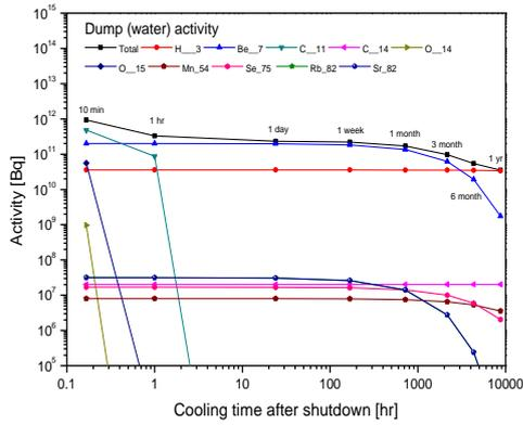
Fig. 6. Activities in the water beam dump according to the cooling time after an irradiation of 3000 hours
