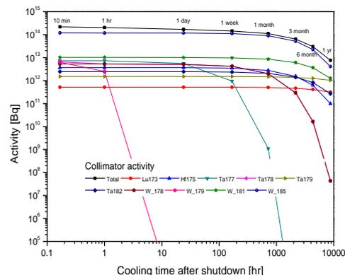
Fig. 3. Activities in the collimator according to the cooling time after an irradiation of 3000 hours
