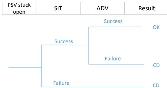
Figure 4 Simplified event tree of POS2 PSV stuck open
