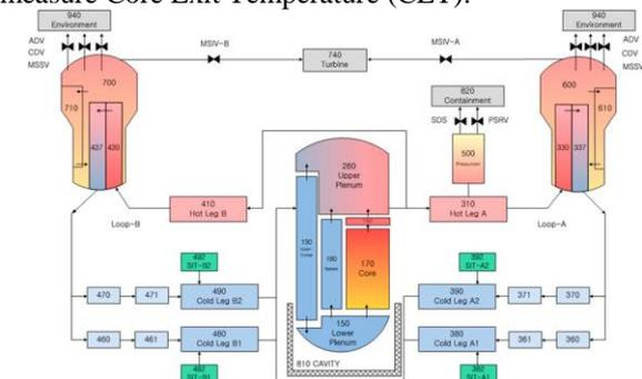
Fig 1. MELCOR nodalization
