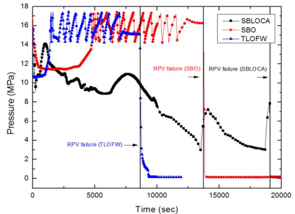
Fig 3. RCS pressure for SBLOCA, SBO and TLOFW
