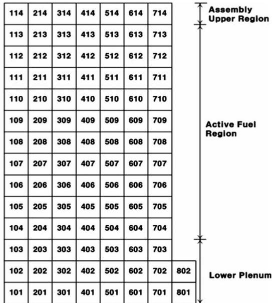
Fig 2. MELCOR nodalization for core
