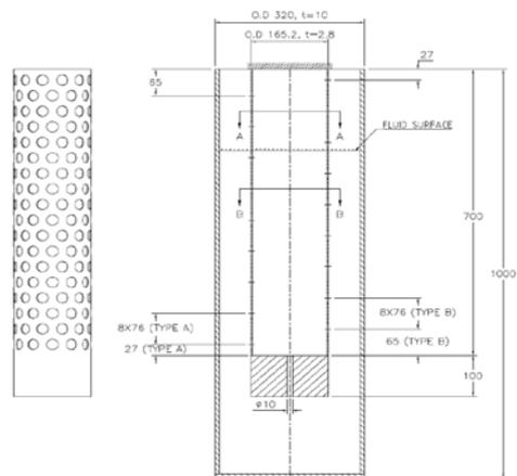
Fig. 1. Dynamic characteristic test model for a cylindrical structure with flow holes
