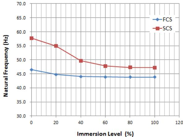
Fig. 4. Comparison of test and analysis results for the natural frequency of the 1<sup>st</sup> bending mode with respect to immersion level.
