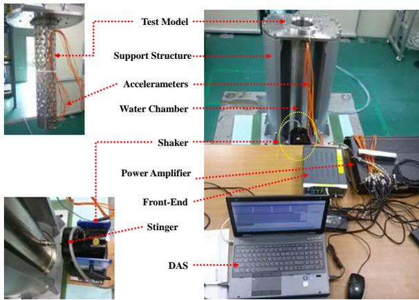
Fig. 2. Test facility of dynamic characteristic tests for a perforated cylindrical structure submerged in water chamber.
