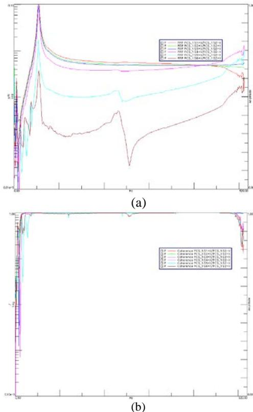
Fig. 3. (a) Frequency response function and (b) coherence function for the FCS test model in an air condition.
