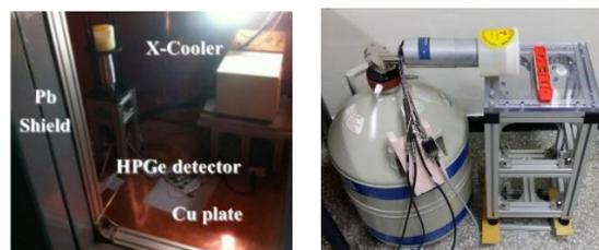
Fig.2. Experimental instruments and detection geometry
