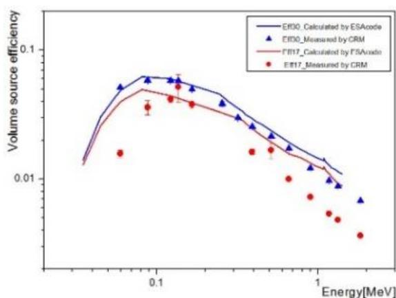
Fig.3. Comparison of efficiency curve between calculation and measurement
