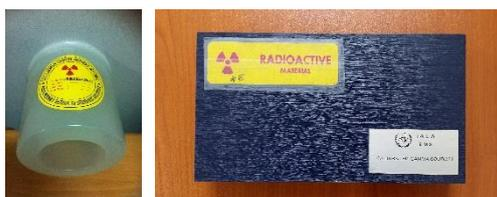
Fig.1. The KRISS CRM volume source and IAEA standard point source
