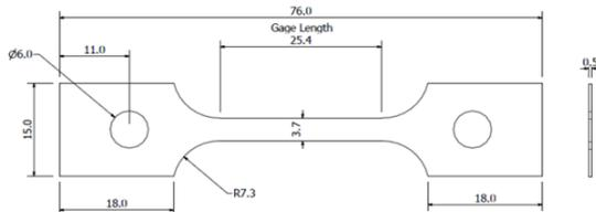
Fig. 1. Tensile specimen geometry
