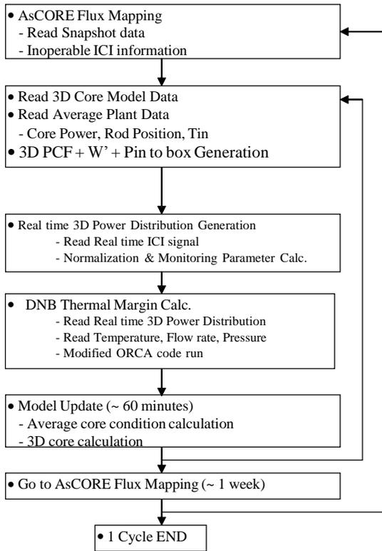
Fig. 6. The flow chart of OASIS program for plant operating simulation.
