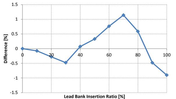
Fig. 5. Fq difference for lead bank insertion at BOC.
