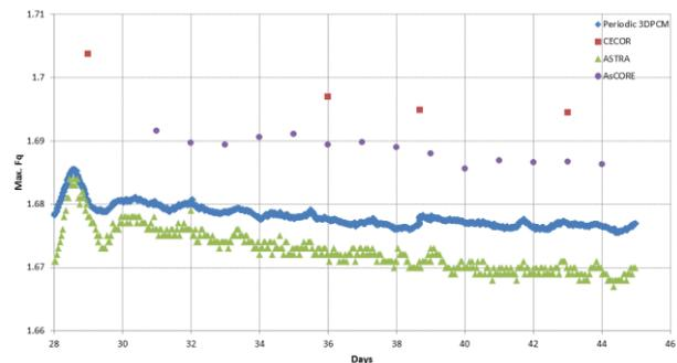
Fig. 9. Fq at BOC HFP operation of a commercial OPR1000 plant in region 4.
