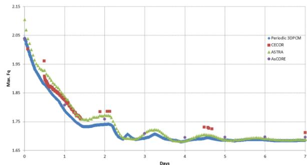
Fig. 8. Fq during the power ascending for a commercial OPR1000 plant in region 1.
