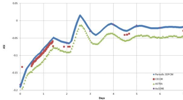
Fig. 10. ASI during the power ascending for a commercial OPR1000 plant in region 1.
