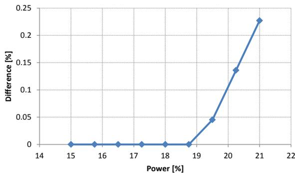
Fig. 2. Fq difference for power increasing operation.
