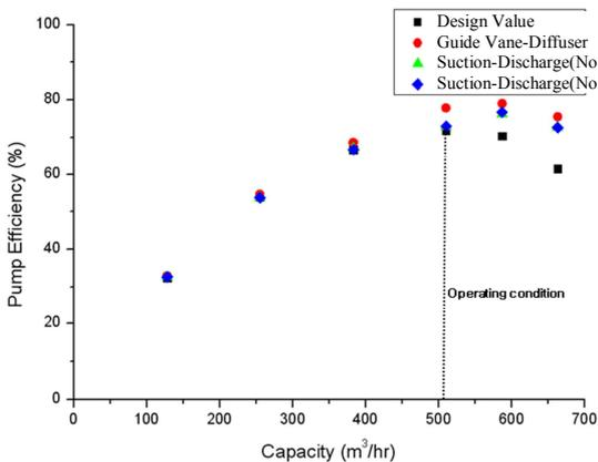
Fig. 4 Curve for efficiency of model pump
