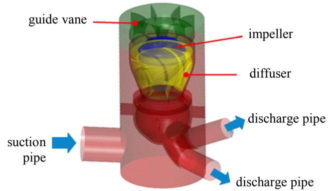
Fig. 1 Schematics of fluid domain in model pump
