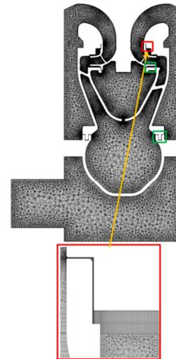
Fig. 2 Numerical grid of fluid domain
