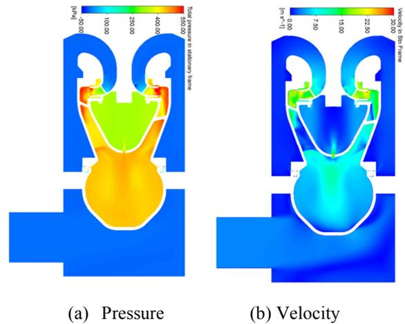
Fig. 5 Predicted pressure and velocity distribution
