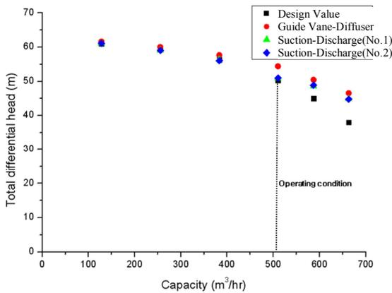
Fig. 3 Curve for head and capacity of model pump
