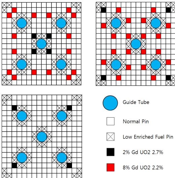
Fig. 1. Assembly Configurations
