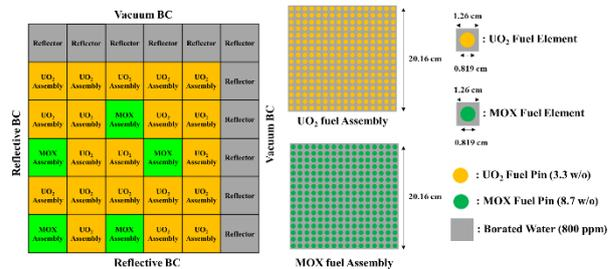
Fig. 3. Two-dimensional continuous-energy thermal reactor test problem
