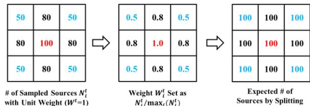
Fig. 2. Example of source splitting in a problem consisting of 9 local domains with vacuum boundary condition
