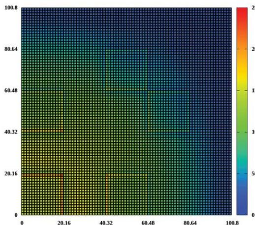
Fig. 4. Pin-power distributions of two-dimensional thermal reactor test problem
