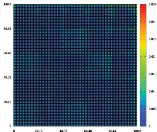
Fig. 6. Relative sample standard deviation of pin-power distributions in Case 2
