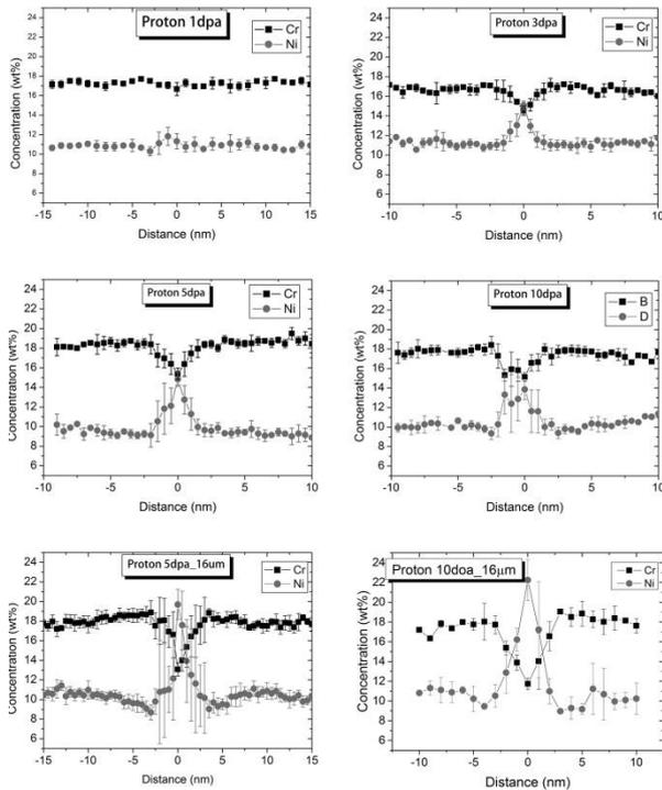
Fig. 2 Cr and Ni concentration profiles at a grain boundary
