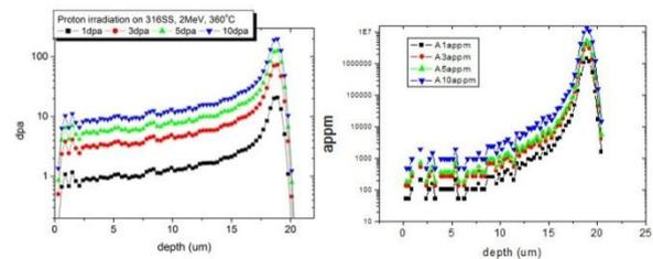
Fig. 1 Radiation damage profiles and implanted H (Proton) by calculation of SRIM code
