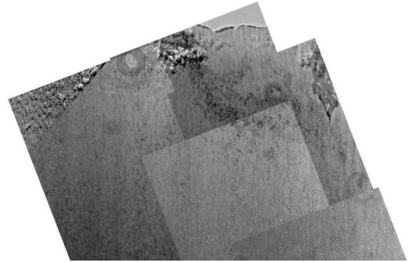
Fig. 3 The formation of cavity in the proton irradiated austenitic stainless steel
