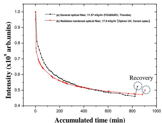
Fig. 2. Variation of transmission rate by high level gamma-ray
