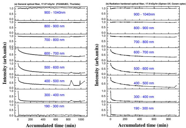
Fig. 3. Transmission rate variation of each wavelength of optical fibers by high level gamma-ray (a) Thorlabs FG365UEC, (b) Ceram optec Optran UV.
