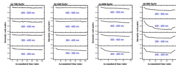
Fig. 5. Variation of transmission rate in wavelength range of 300 to 500 nm by dose rate (a) 180 Gy/hr, (b) 540 Gy/hr, (c) 600 Gy/hr, (d) 680 Gy/hr.
