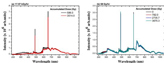
Fig. 4. Transmission rate of Thorlabs FG365UEC by dose rate variation (a) 17.57 kGy/hr, (b) 58 Gy/hr.
