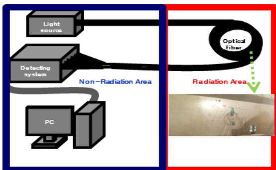
Fig. 1. Experiment diagram.
