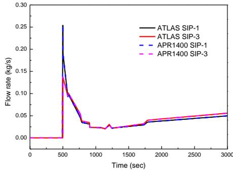
Fig. 4. Safety Injection Pump flow rate
