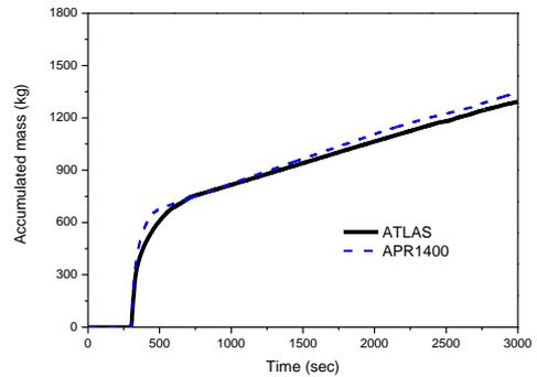
Fig. 7. Accumulated break flow rate.
