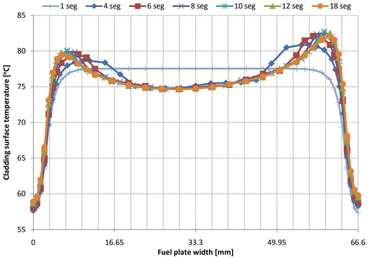
Fig.4. Wall temperature distribution with various numbers of segments
