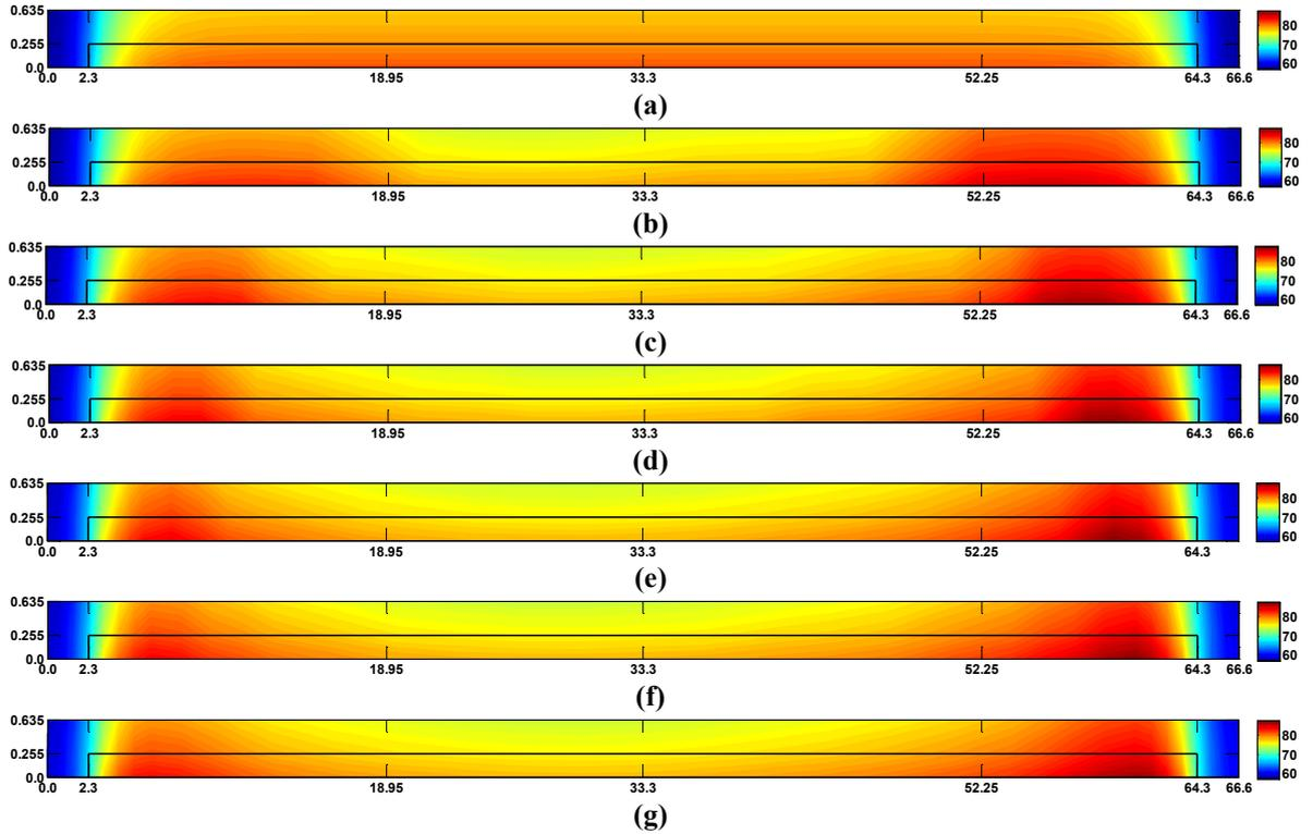
Fig.3. Fuel temperature with transverse power distribution: (a) 1 segment, (b) 4 segments, (c) 6 segments, (d) 8 segments, (e) 10 segments, (f) 12 segments, and (g) 18 segments
