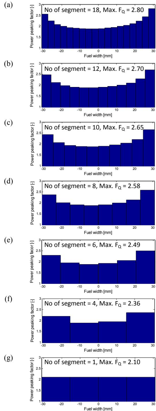
Fig.2. Transverse power distribution with segments
