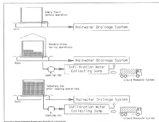
Fig. 1. Separative Water Collection System in the surface disposal facility (l'Aube Facility)
