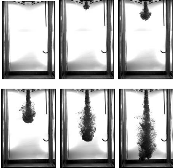
Fig. 2. Jet breakup snap shot every 0.1 s ( D_{jet} = 50 mm, V_{jet} = \sim 1.5 m/s)
