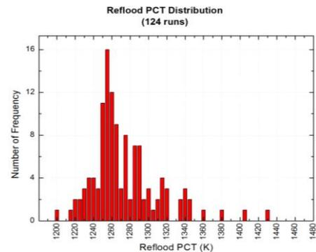
Fig. 4. Frequency of Reflood PCT, K
