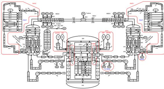
Fig. 1. MARS-KS APR+ Nodalization
