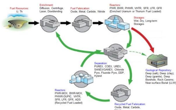
Fig. 1. Typical nuclear fuel cycle flow and lists of potential options for each fuel cycle step.
