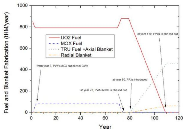
Fig. 6. Fresh fuel fabrication rate.
