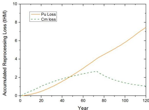
Fig. 8. Pu and Cm losses in reprocessing.
