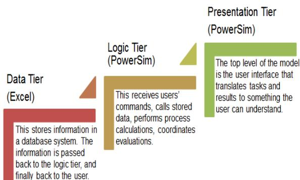
Fig. 2. Overall structure of the developed program for dynamic nuclear fuel cycle analysis.
