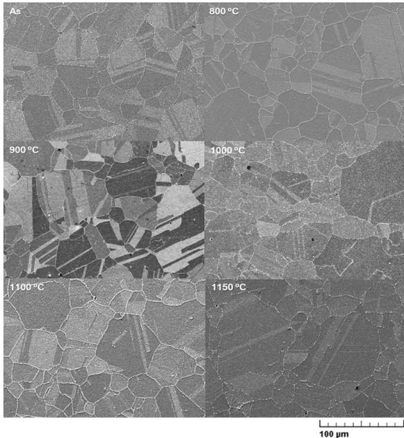
Fig. 1. SEM images of Alloy 690 quenched after 20 minutes of solution heat treatment at the range of 800~1150°C
