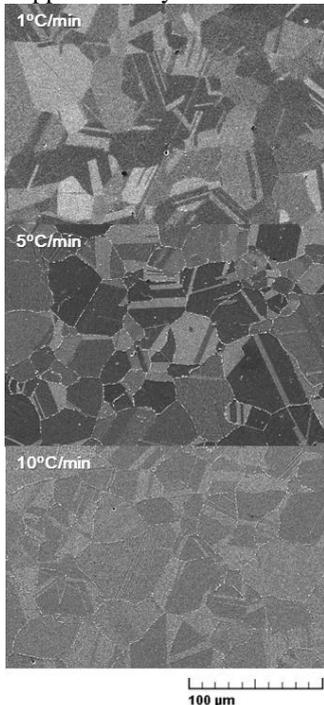
Fig. 2. SEM images of Alloy 690 quenched after 20 minutes of solution heat treatment at 1150°C, cooling to 800°C, which is the medium temperature, with the cooling rate of 1°C /min, 5°C /min, 10°C /min and 100 minutes of aging heat treatment.
