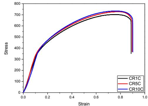
Fig. 3. Tensile test in relation to the cooling rate.
