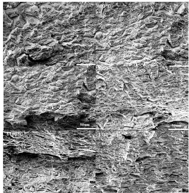
Fig. 4. SEM images of SEM fracture surface after tensile test of Alloy 690.
