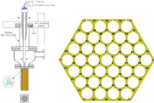
Fig. 3. Schematic of the sampling probe and numbering of subchannels.
