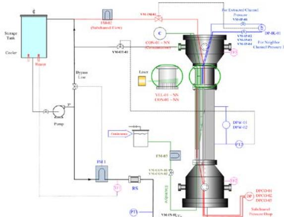
Fig. 1. Schematic drawing of the test loop (FIFFA).
