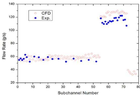
Fig. 4. Subchannel flow rates in experiments and CFD analysis ( $Re = 37,110$ ).
