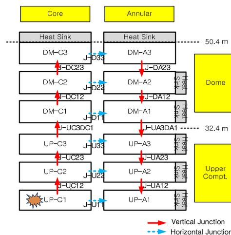
Fig. 1 CAP Input Nodalization Model
