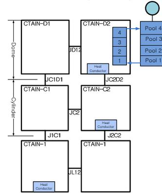
Fig. 4 Nodalization of SMART
