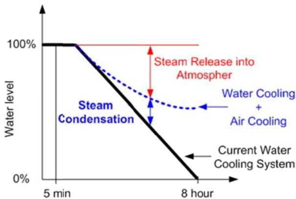
Fig. 3 Steam Condensation vs. Steam Discharge in an Air-Cooling Heat Exchanger
