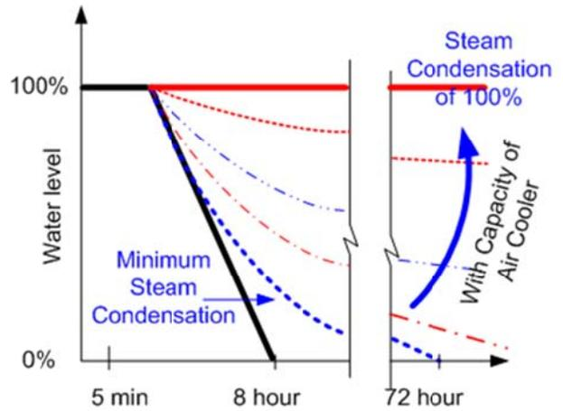
Fig. 4 Water Level vs. Capacity of an Air-Cooling Heat Exchanger for 72-hour Operation
