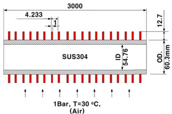
Fig. 5 Dimension of Finned Tube
