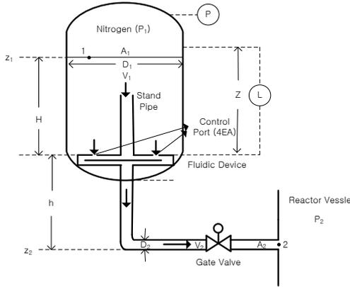
Fig. 1 Schematic Diagram of SIT Performance Verification
