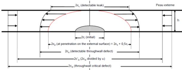
Fig. 1. Change of the semi-elliptical crack shapes after penetration
