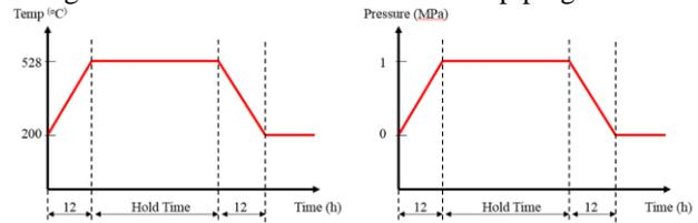
Fig. 3. Operation condition of IHTS piping
