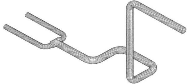
Fig. 2. Finite element model for IHTS piping
