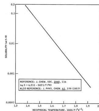
Fig. 1 Solubility of hydrogen vs. temperature in sodium[3]
