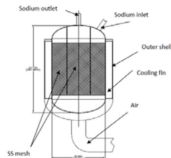
Fig. 2 Cold Trap assembly
