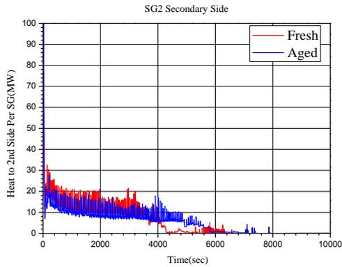
Figure 2 Heat Transfer Through SG U-tubes
