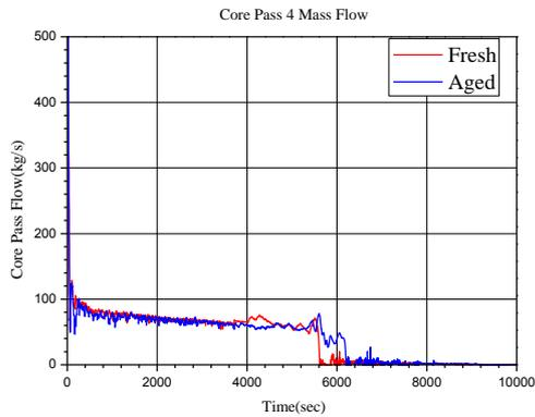
Figure 3 Core Pass Flow
