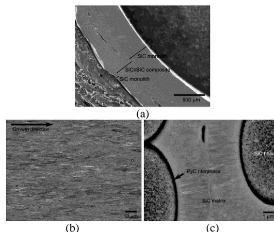
Fig. 1. Typical microstructure showing (a) the SiC triplex tube fabricated by the chemical vapor processes, (b) SiC monolith, and (c) Tyranno SA3-reinforced SiC<sub>f</sub>/SiC composite.
