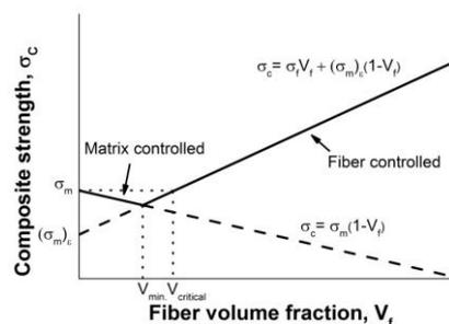
Fig. 2. Relationship between composite strength and fiber volume fraction.
