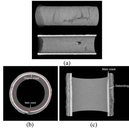
Fig. 4. Micro-CT images of a SiC triplex tube after failure.
