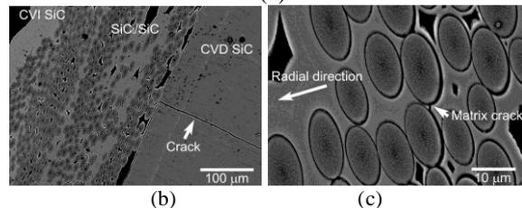
Fig. 5. (a) Hoop stress vs. radial displacement curve of a SiC triplex tube and (b) microstructure of the SiC triplex tube showing a crack in a SiC inner layer and (c) matrix cracks in a SiC/SiC composite layer.
