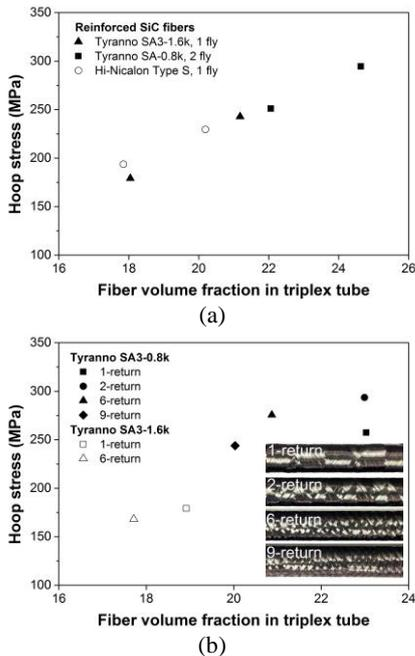
Fig. 3. Hoop stresses of the SiC triplex tubes as a function of the fiber volume fraction: (a) 1-return of the winding pattern and (b) four phase winding patterns
