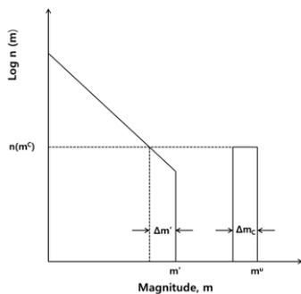
Fig. 3. Generalized frequency magnitude density function for the characteristic earthquake model [4]
