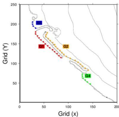
Fig. 7. The group of wave height sampling points (G1:front of intake, G2:front of breakwater, G3:left side of breakwater, G4:right side of breakwater) [5]
