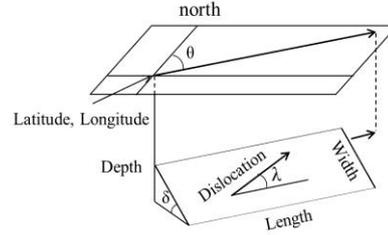
Fig. 4. Definition of fault parameters [5]
