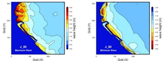
Fig. 6. The maximum and minimum wave height distribution of the E3 fault source [5]
