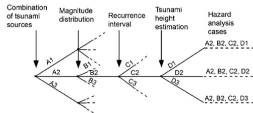
Fig. 1. Outline of a logic-tree approach used for the tsunami hazard analysis [1]
