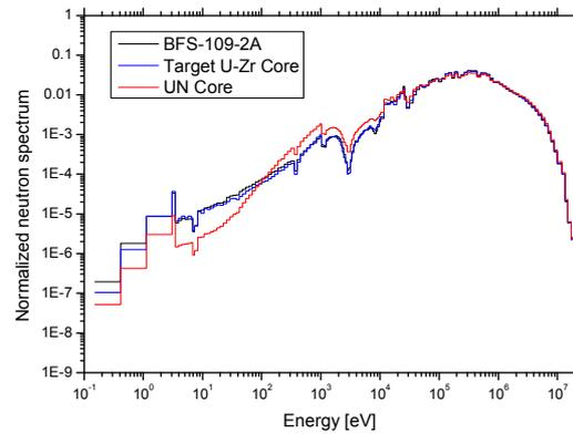
Fig. 1. Neutron spectrums in the central core region
