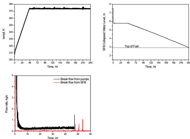
Fig. 4 Results of pipe rupture in the SFB for SFB normal operation
