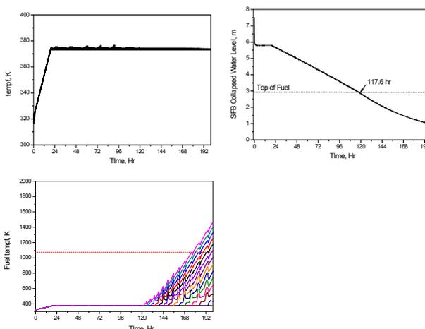
Fig. 6 Results of pipe rupture in the SFB for SFB abnormal operation
