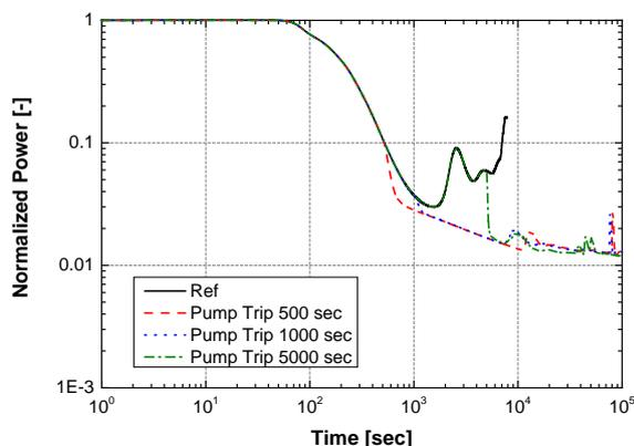
Fig. 11 Normalized power during the ULOHS event for different trip times of the primary pumps
