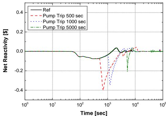
Fig. 10 Net reactivity during the ULOHS event for different trip times of the primary pumps
