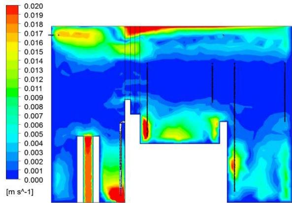
Fig. 5. Velocity distribution when HWLS inlet  $T_H = 40$  °C.
