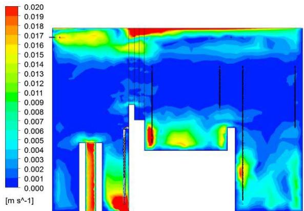
Fig. 6. Velocity distribution when HWLS inlet  $T_H = 45$  °C.
