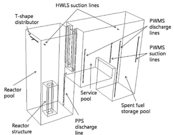
Fig. 1. Basic design of the on-going KIJANG research reactor.
