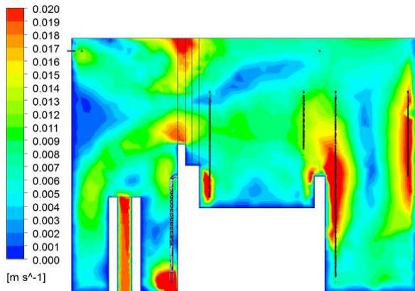
Fig. 3. Velocity distribution when HWLS inlet  $T_H = 35$  °C.
