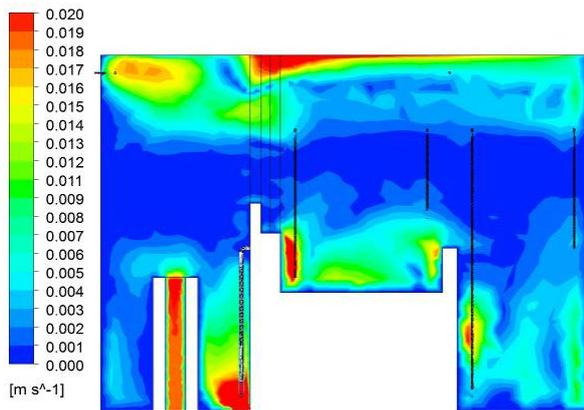
Fig. 4. Velocity distribution when HWLS inlet  $T_H = 37.5$  °C.
