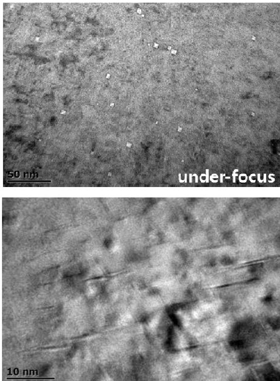
Figure 5 Plate-like precipitates on a 5 dpa proton irradiated sample
