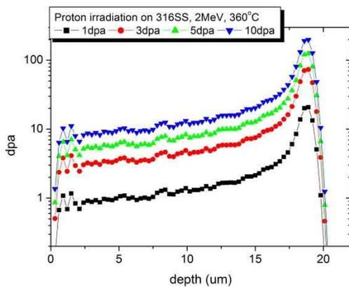
Figure 3 Calculation of proton irradiation profile on 316 SS
