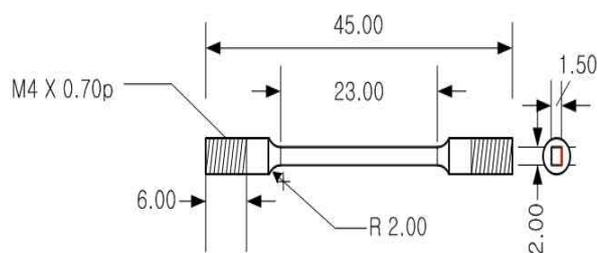
Figure 2 Schematic of IASCC initiation test specimen
