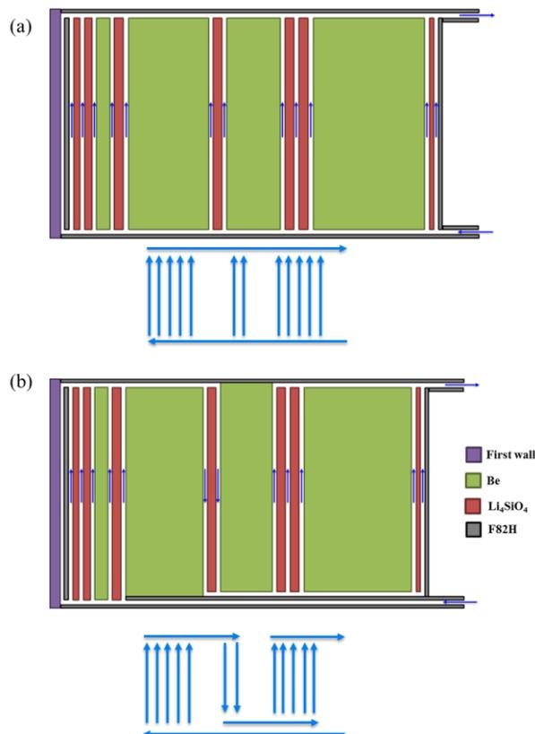
Fig. 2. Two flow line concept for breeding blanket
