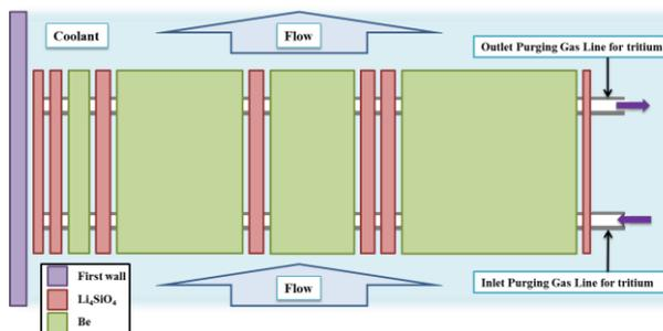
Fig. 1. Plate-type breeding blanket concept K-DEMO
