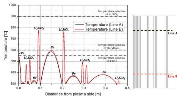
Fig. 3. Temperature distribution in breeding blanket
