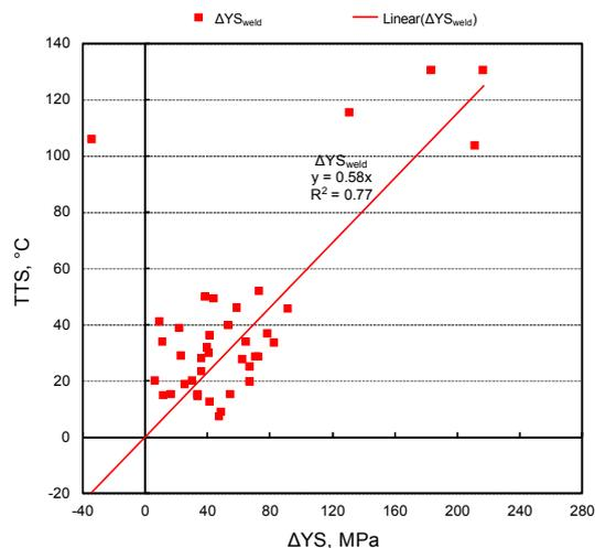
Fig. 4. Plots of  $\Delta YS$  versus TTS: weld metal. Kori-1 data points are included (TTS > 100°C).
