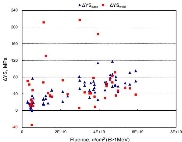
Fig. 3. Changes in yield strength of the base metal and weld metal of Korean surveillance data with neutron irradiation
