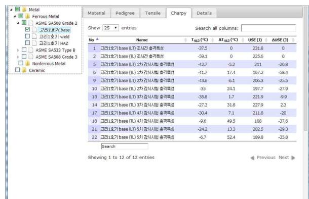
Fig. 2. Charpy impact test results of the Kori-1 unit base metals.
