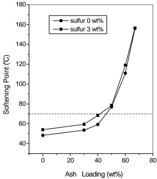
Fig. 1 Influence of sulfur on the softening point of waste forms
