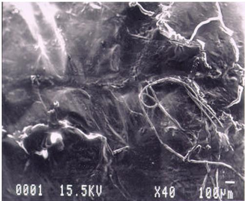
Fig. 3 Scanning electron micrograph of the matrix (bitumen + waste PE)
