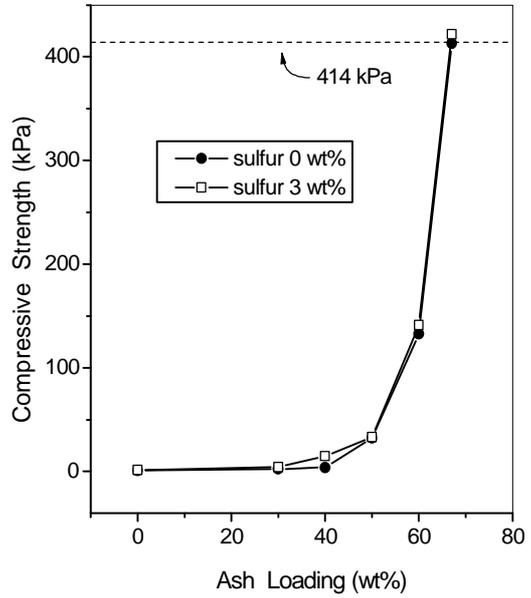
Fig. 2 Influence of sulfur on the compressive strength of waste forms (deformation 10%)
