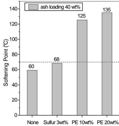
Fig. 6 Influence of the additives on the softening point and compressive strength at ash loading 40wt%
