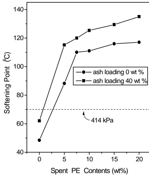
Fig. 4 Influence of spent PE contents on the softening point of waste forms
