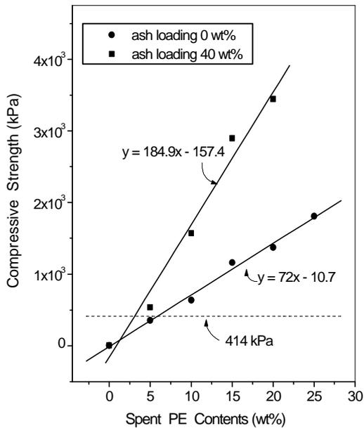
Fig. 5 Influence of spent PE contents on the compressive strength of waste forms (deformation 10%)
