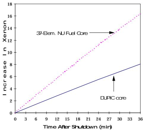
Fig.3 Xenon Transient 30 Minutes After Shutdown
