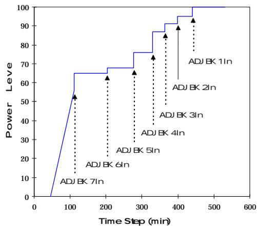
Fig.4 Reactor Power Level vs. Time in Restart from Short Shutdown
