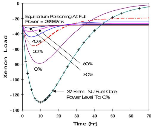
Fig. 6 Variation Of Xenon Load Following Step Power Reductions From Full Power
