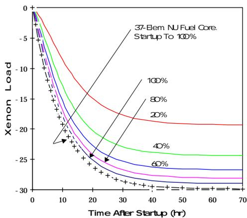
Fig. 5 Xenon Transients After Startup From Long Shutdown To Various Local Power Levels
