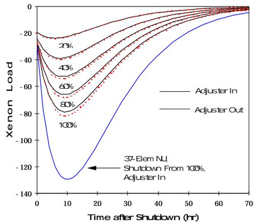
Fig.2 Xenon Load After Shutdown From Various Power Level
