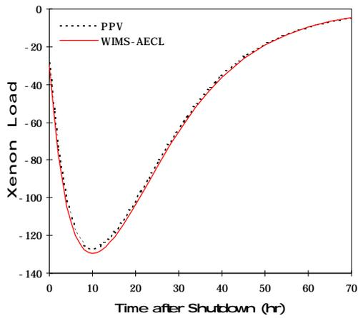
Fig. 1 Xenon Load After Reactor Shutdown From 100% Power (37- Element NU Fuel Core)
