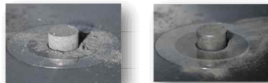
Fig. 3. Green compacts of metallic uranium powder with the addition of 30 vol.% of molybdenum (left) and chromium (right).
