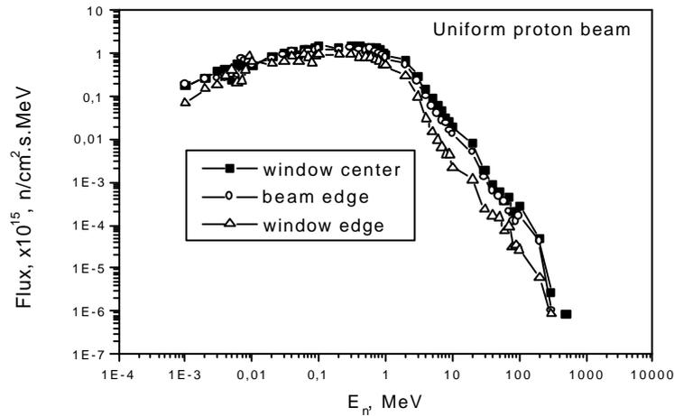
Figure 2. Neutron energy spectrums for uniform proton beam.
