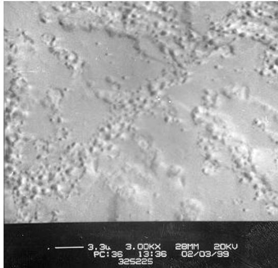
Fig. 3. Back-scattered scanning electron image of atomized U-10wt.%Mo microplate at 70at.% burnup.
