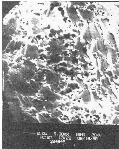
Fig. 1. Scanning electron micrographs for U-10wt.%Mo microplates at 40at.% burnup;
