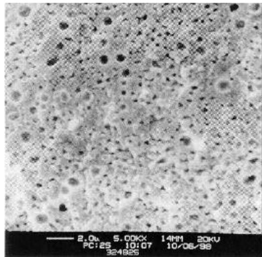
Fig. 2. Scanning electron micrographs for U-10wt.%Mo microplates at 70at.% burnup;
