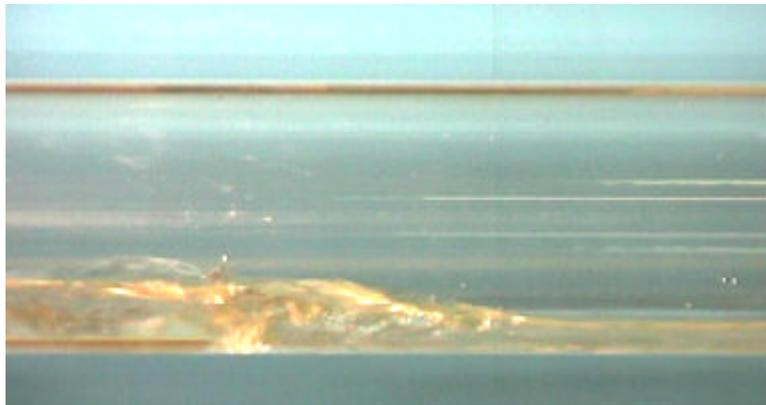
**Fig. 5 Hydraulic Jump in the Horizontal Pipe ( $j_L^* 0.5 < 0.2$ )**
