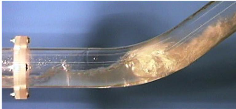
Fig. 6 Water Hold Up at the Bend When the CCFL Occurs ( $j_L^{*0.5} < 0.2$ )
