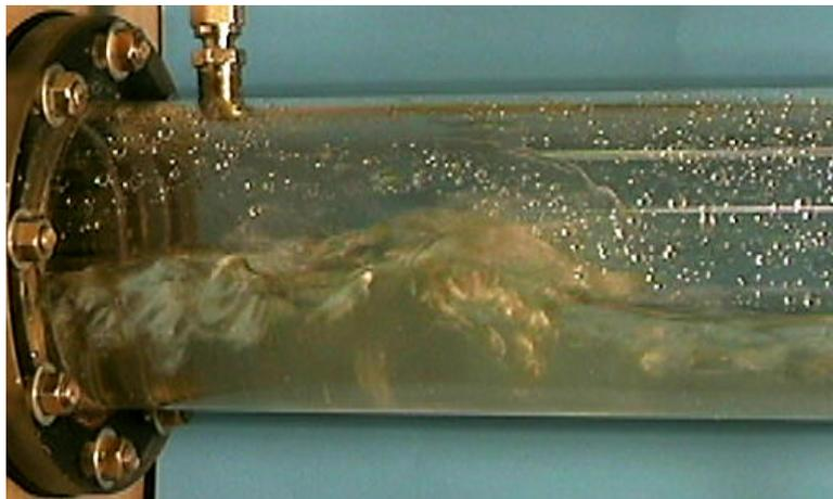
Fig. 7 The Large Roll Wave Formation at the Outlet of Water ( $j_L^{*0.5} = 0.2 \sim 0.4$ )
