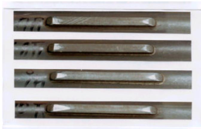
2. Typical Wear Marks on Bearing Pads
