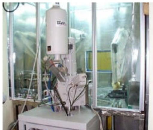
Fig. 4. SEM in the Shielded Glove Box.
