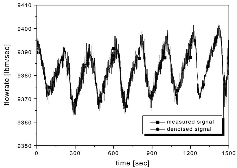
Fig. 5. Wavelet Denoising of the Hot-Leg Flowrate.
