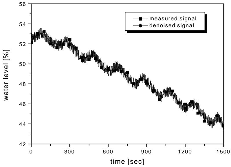
Fig. 4. Wavelet Denoising of the Pressurizer Water Level.
