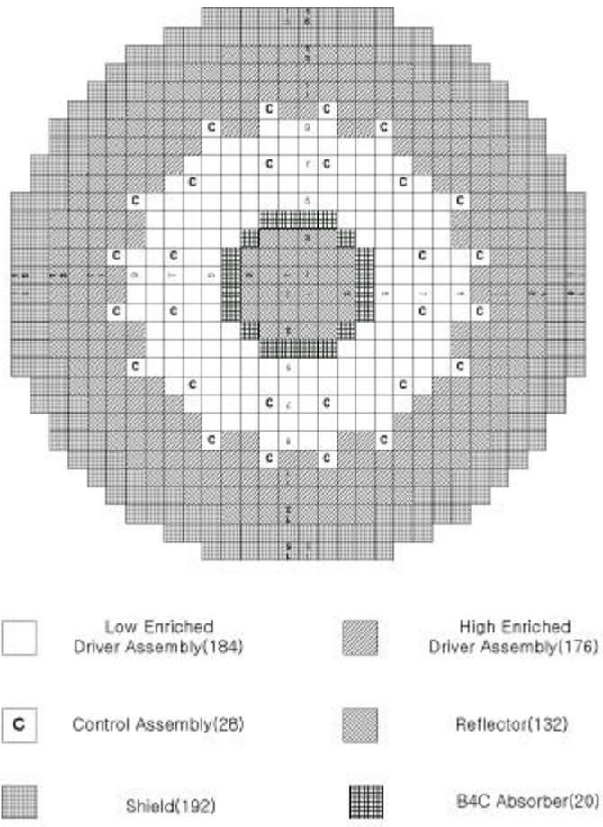
Figure 2. Cross sectional view of reference core
