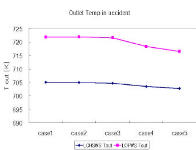
Figure 7. Outlet Temperature in LOHSWS and LOFWS.
