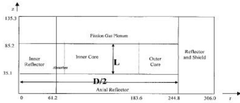
Figure 1. Core side configuration of reference design.
