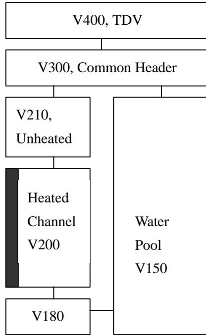
Fig. 2 RELAP5 Node-Flow Path Network
