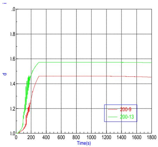
Fig.12 Void fraction in the flow channel
