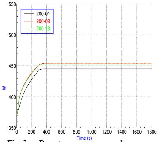
Fig.3 Reactor vessel wall void fraction in the flow channel
