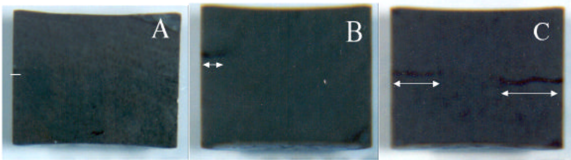
Fig. 5. Crack shapes of simulated DUPIC fuel and simulated spent fuel :
