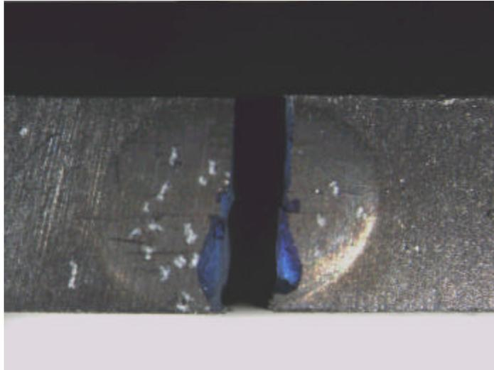
Fig. 4. Top surface of fractured hydride blister.
