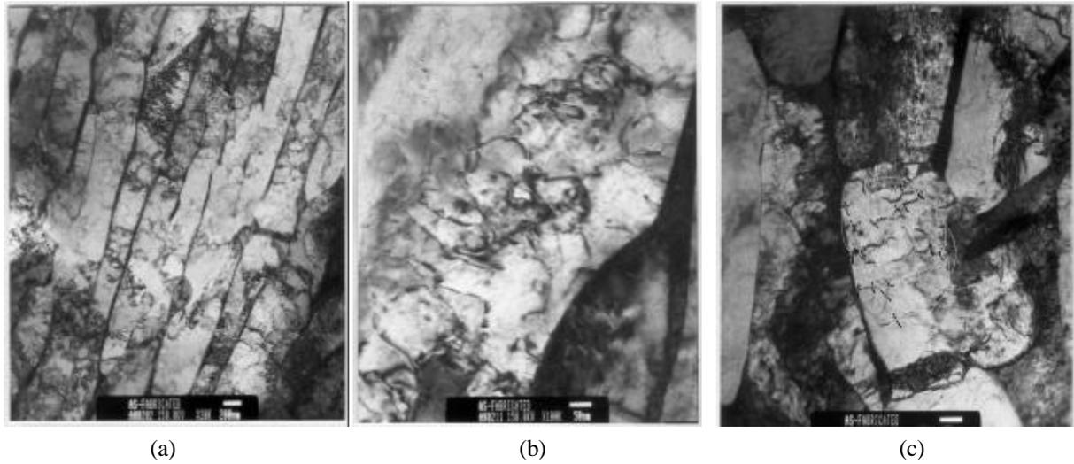
Fig. 1. Microstructures of the unirradiated Zr-2.5Nb tube made of the same lot as that of W1M11 tube: (a) grain structures, (b)  $\langle a \rangle$  component dislocations and (c)  $\langle c \rangle$  component dislocations.
