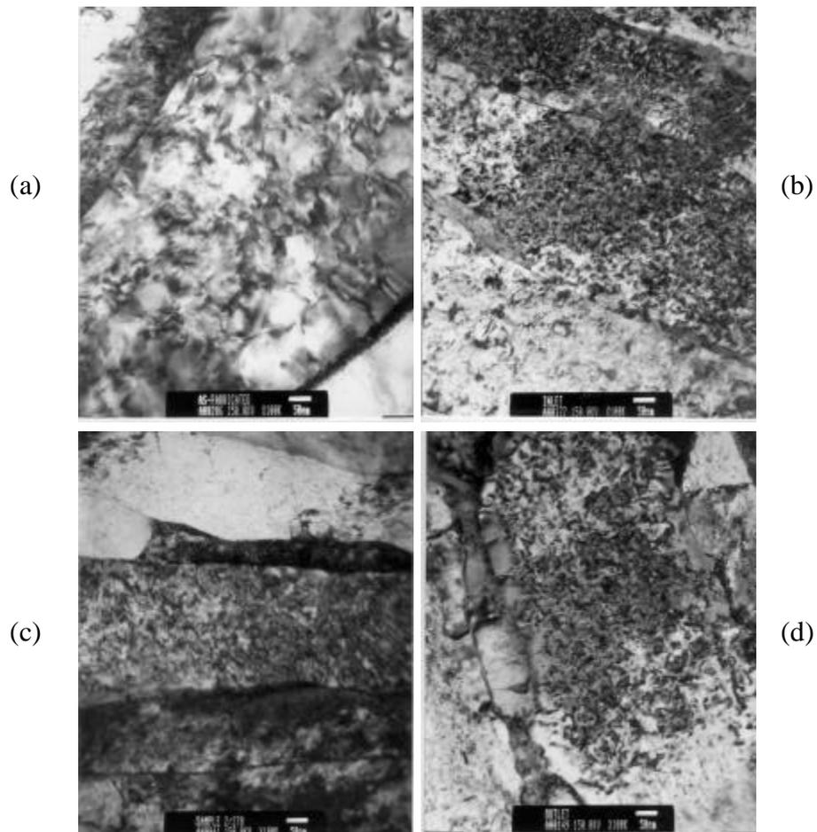
Fig. 2. Evolution of  $\langle a \rangle$  type dislocations with irradiation in the W1M11 pressure tube: (a) before irradiation and (b-d) after irradiation – (b) the inlet, (c) the middle and (d) the outlet.
