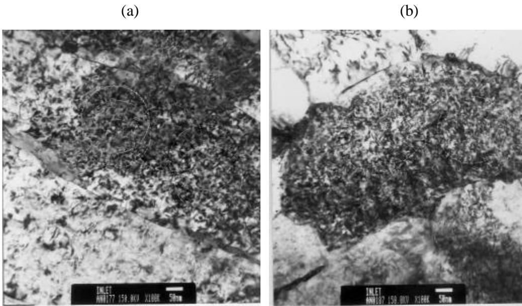
Fig. 3. <a> type dislocation loops on the inlet ring of the W1M11 tube irradiated to  $8.9 \times 10^{25} \text{ nm}^{-2}$ .
