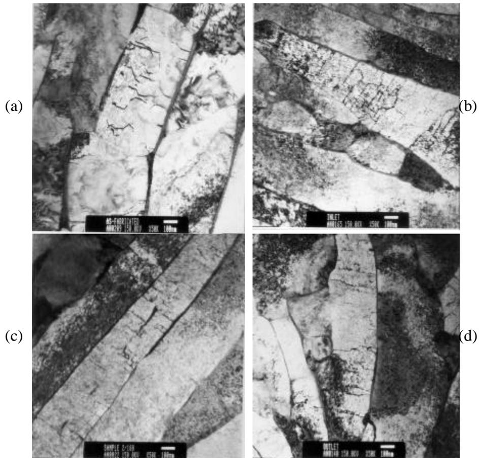
Fig. 4. Typical <c> component dislocations in the W1M11 tube irradiated to  $8.9 \times 10^{25} \text{ nm}^{-2}$  along with those of the preirradiated tube: (a) preirradiated tube, (b) the inlet, (c) the middle and (d) the outlet of the W1M11 tube.
